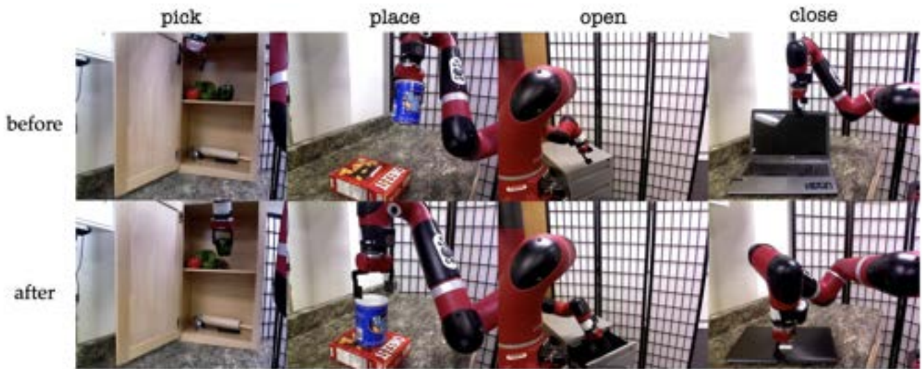
Figure 5.3: Robot demonstrations recorded in the lab illustrating snapshots before and after a robot executing the pick , place , open , close actions.
