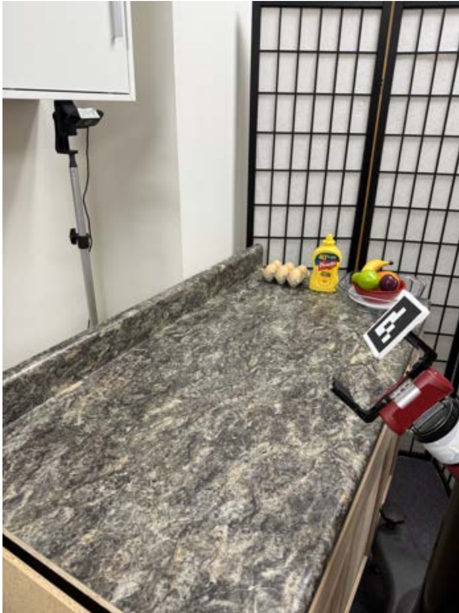
Figure 6.2: The hand-eye calibration system consisting of an HD camera fixed on a tripod and the Sawyer robot with an attached ArUco marker on its right_gripper_r_finger_tip link.
