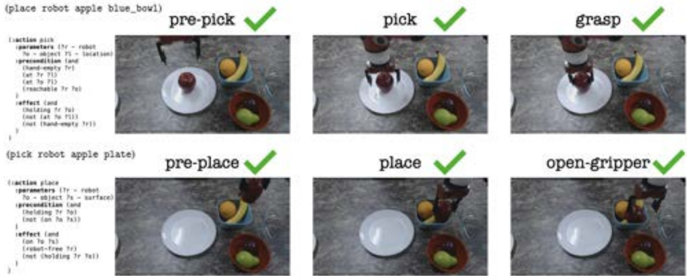
Figure 5.8: Successful action execution by visually grounding PDDL action preconditions and effects.
