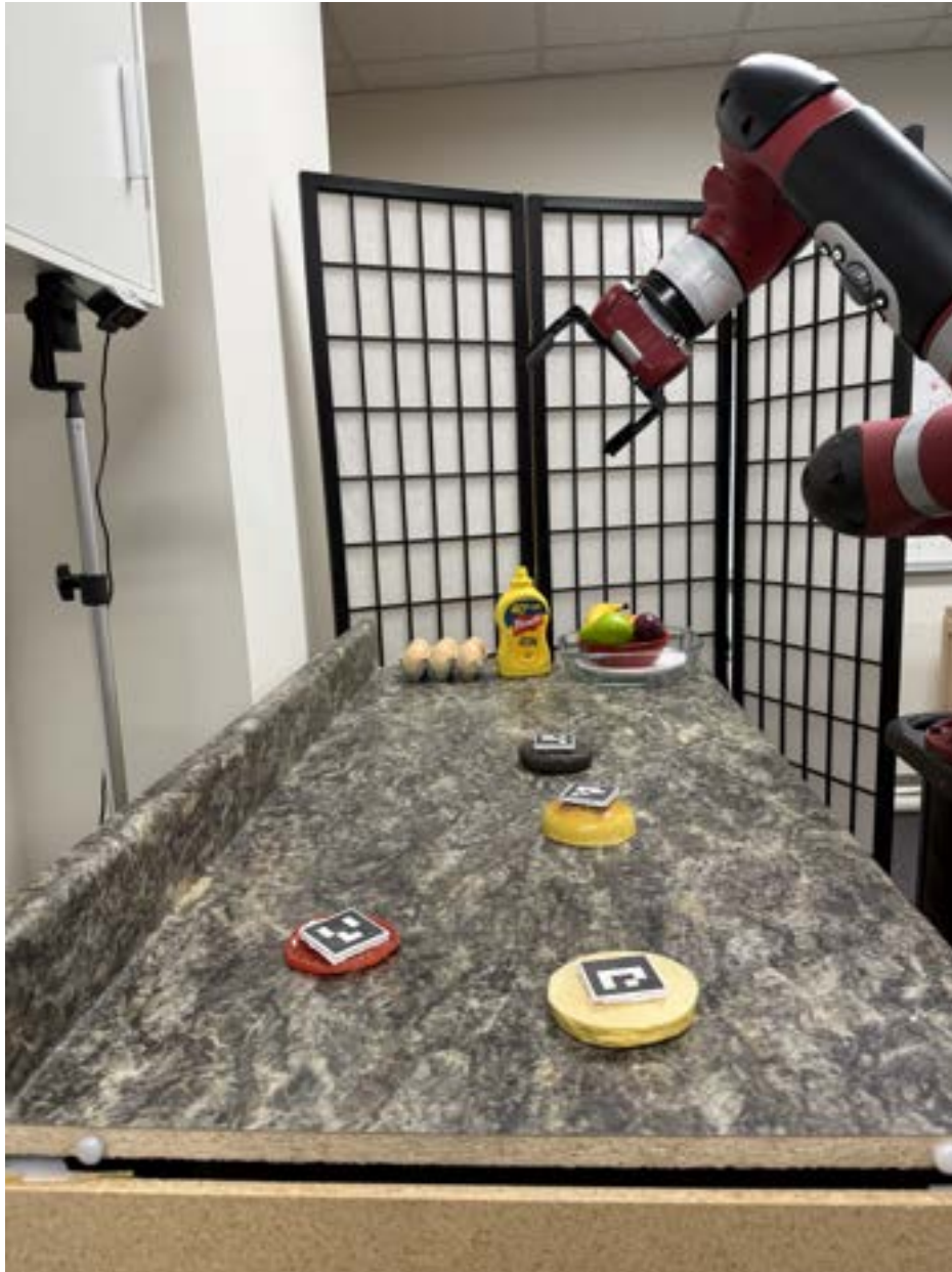
Figure 6.7: The initial state of the scene featuring the Sawyer robot-HD camera hand-eye calibrated system and the ingredients, randomly placed on the kitchen counter.
