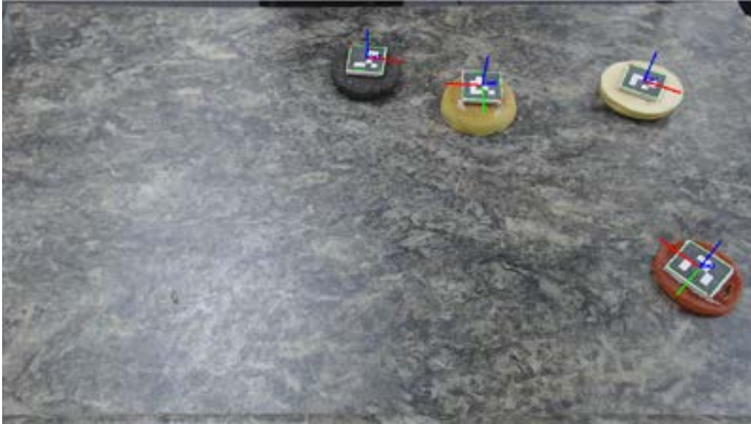
Figure 6.4: Transforms of the markers tracked through the aruco_detect node and published through the fiducial_to_tf node in rviz.
