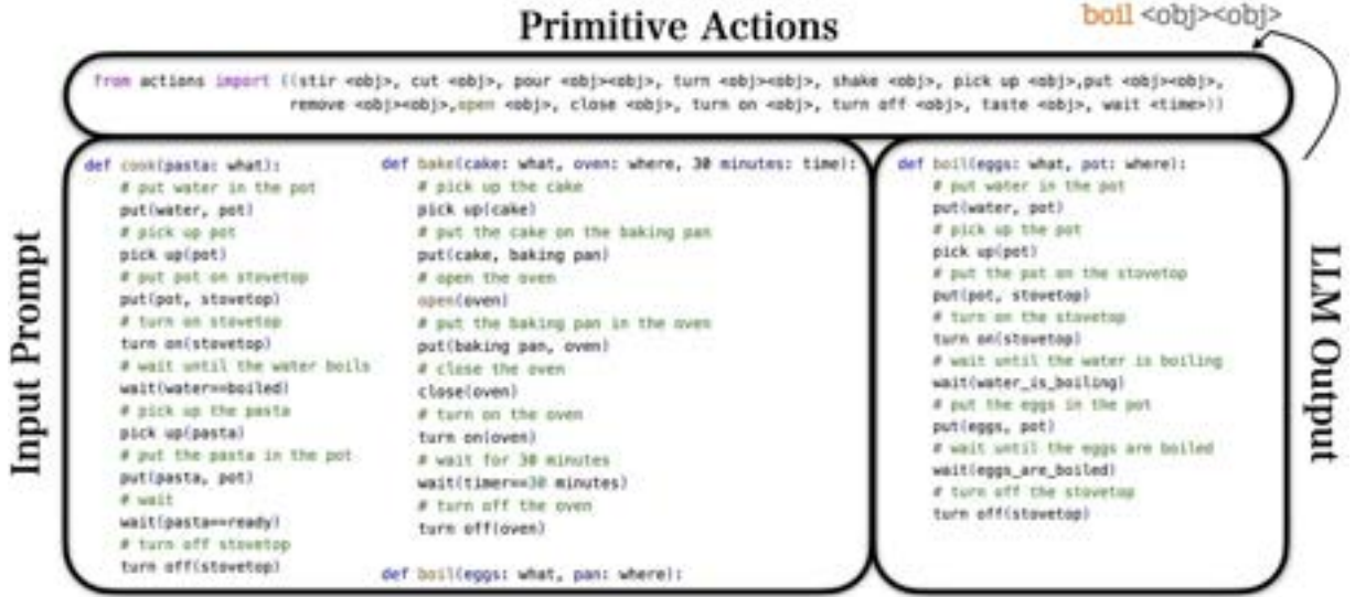
Figure 3.4: Inspired by ProgPrompt [3], Cook2LTL uses an LLM prompting scheme to reduce a high-level cooking action (e.g. boil eggs) to a series of primitive manipulation actions. The prompt consists of an import statement of the primitive action set and example function definitions of similar cooking tasks. The key benefit of using this paradigm is that it constrains the output action plan of the LLM to only include subsets of the available primitive actions. We extend this prompting scheme by reusing derived LLM policies. In this case, the action boil is added to future import statements in the input prompt, enabling the model to invoke the derived boil function which is now considered given to the system.
